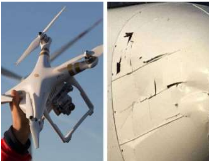
Figure 3 - A Drone crash with an aeroplane in Mexico (A Drone Hit A Boeing 737 In Mexico, 2018)
